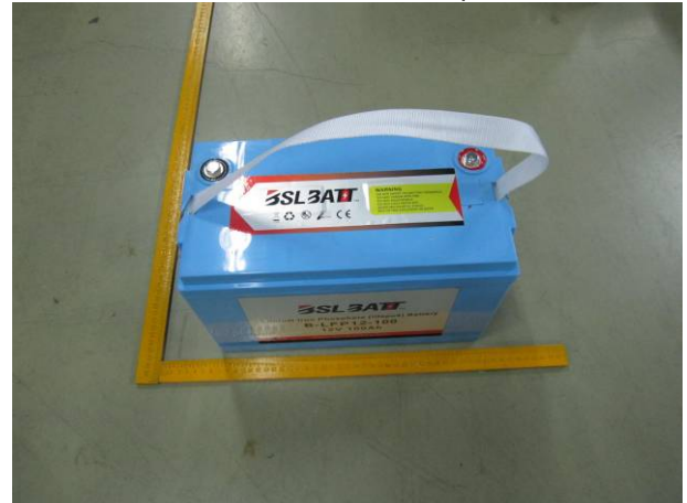
电池/ Battery(B-LFP12-100 12,8V 100Ah 1280Wh)
